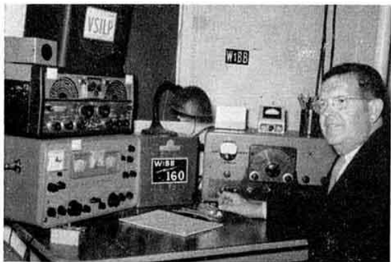
W1BB/I 160m DX station in a stone house beside the Atlantic Ocean. The aerial is an inverted-V with the apex 260 ft. above a salt water ground-plane, and the equipment consists of a Valiant transmitter, and a Hammarlund HQ170 receiver with a Hallicrafters SX100 auxiliary receiver.
