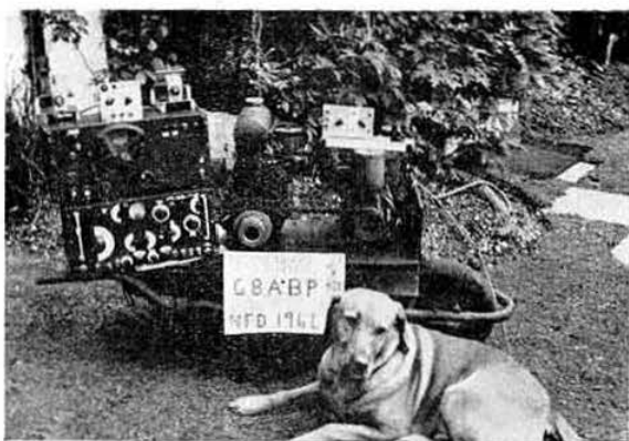
The Loughton and District Radio Club equipment, with operator G8AB/D (Rusty). All the apparatus including the generator was home constructed, and consisted of a double superhet; v.f.o.-b.a.-f.d.-p.a. transmitter; aerial tuning unit and aerial switching unit, which fed two 7 Mc/s collinear arrays and a ground plane.
